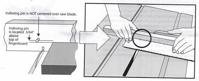
Prior to slotting, true one or both edges of the blank fingerboard. Attach the fret scale template to the back of the fingerboard with double-stick tape. Choose one of the two scales, and be sure the notched edge you're using is flush to the trued edge of the fingerboard. The edges of the fingerboard and template together will rest against the miter fence.
