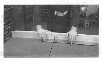
**Optional Shooting Board:** For the most accurate work, build a "shooting board," a sliding platform with a long fence and two guides fastened to the bottom that slide through both the right and left slots on the table-saw top. This makes for square, accurate cross-cutting.
